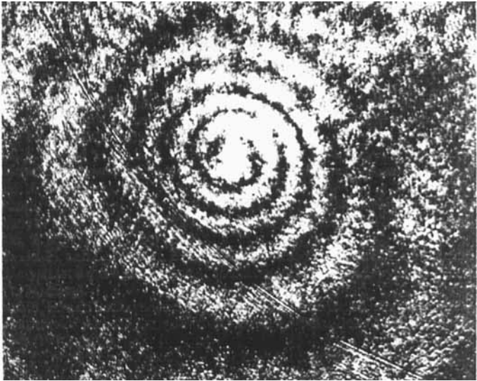
FIGURE 11 Reconstructed image from a double-exposed hologram. The observed interference fringes form a spiral.
